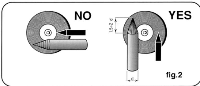
**CAUTION:** HOT FLYING METAL PARTICLES can injure persons, start fires and damage equipment. TUNGSTEN CONTAMINATION can lower the welding quality.
