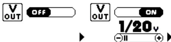
The factory default mode is OFF meaning that there is no voltage between outlet pins 5 (-) and 6 (+).
