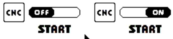
By setting this function on ON you enable START mode from the CNC relative to pins 3 and 4 of the AMP connector located on the rear of the power source and, at the same time, the manual start located on the machine's front adapter is disabled.
