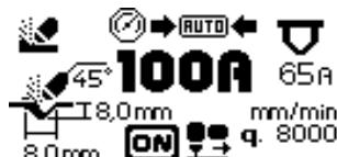
The power source automatically displays the width and depth of the groove that can be achieved with the current values (Pict. 4 Ref. G) at the relative processing speed (Pict. 4 Ref. E) set by the operator, and tells you which nozzle to use (Pict. 4 Ref. F) and the inclination in degrees that the torch needs to be maintained at during forward movement.
