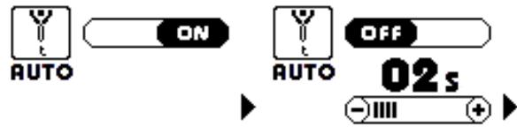
The factory default mode is AUTO ON which allows the power source to automatically and synergically adjust the
