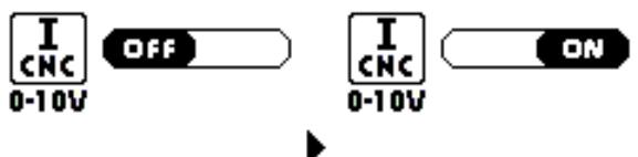
The factory default mode is OFF meaning that there is no chance of adjusting the cutting current remotely between pin 1 (0V) and pin 2 (10V).
