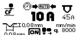
The power source automatically displays the width and depth of the groove that can be achieved with the current values (Pict. 4 Ref. G) at the relative processing speed
