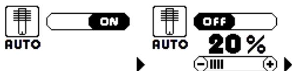
The factory default setting is AUTO ON which allows the power source to interrupt operation independently when electrode and nozzle need replacing. It is nevertheless
