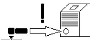
If this picture appears the machine is reporting that either no torch has been connected or an invalid one has been connected.
