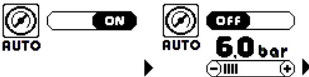
The factory default mode is AUTO ON which allows the power source to maintain the torch's work pressure at the best value, also in the presence of variations of the inlet pressure.
