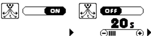
The factory default mode is AUTO ON which allows the power source to automatically and synergically adjust post gas duration based on the mounted torch, the set current value and the selected processing procedure. It is nevertheless possible to set this function on OFF so as to be able to manually adjust post gas duration (within certain pre-set limits).
