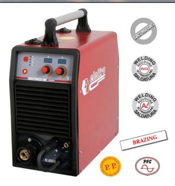
MULTIWELD 186 SYNERGIC is a single-phase multipurpose inverter power source, suitable for welding alternately in MIG/MAG, MMA (stick electrode) and DC TIG ("lift" start) mode. It has a compact design, low weight and offers the possibility to be connected to home mains (3kW) and to generators with a power at least of 4,8 kVA.
