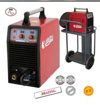
MULTIWELD 236 SYNERGIC is a single-phase multipurpose inverter power source, suitable for welding alternately in MIG/MAG, MMA (stick electrode) and DC TIG ("lift" start) mode. It has a compact design, a low weight and, with a welding current of 220A, allows to weld wires up to a diameter of 1,2mm. It can be connected to generators.
