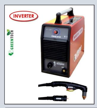
The three-phase power source with inverter technology for metal plasma cutting, **PLASMA 50-23 INVERTER** is characterized by compact design, low weight, easy handling, user-friendliness, cutting high-efficiency on small and medium thicknesses.
